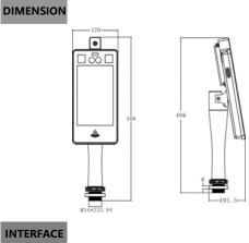
1-Wiegand 2-Alarm out 2 3-RJ45 4-DC12V 5-Alarm out 1+RS485
